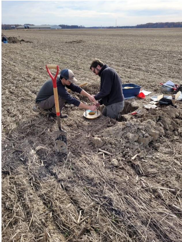
Matt Tucker, SSPL-Findley, OH and Stephen Roecker, SSPL- Indianapolis, IN conducting compliant cavity tests in a satellite pit of the Cobbsfork “new” field.
