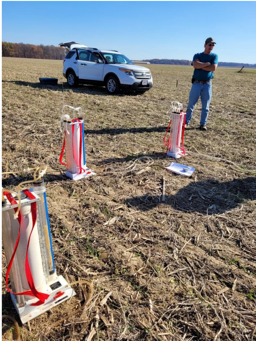
Constant head permeameter (Amoozemeter) set up on “new” Avonburg field
